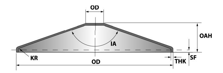
Key: KR-Knuckle Radius IA-Included Angle OD-Outside Diameter SF-Straight Flange THK-Thickness OAH-Overall Height
