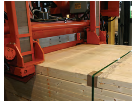
Automatic top and bottom edge protection using flat fibreboard edge protectors
